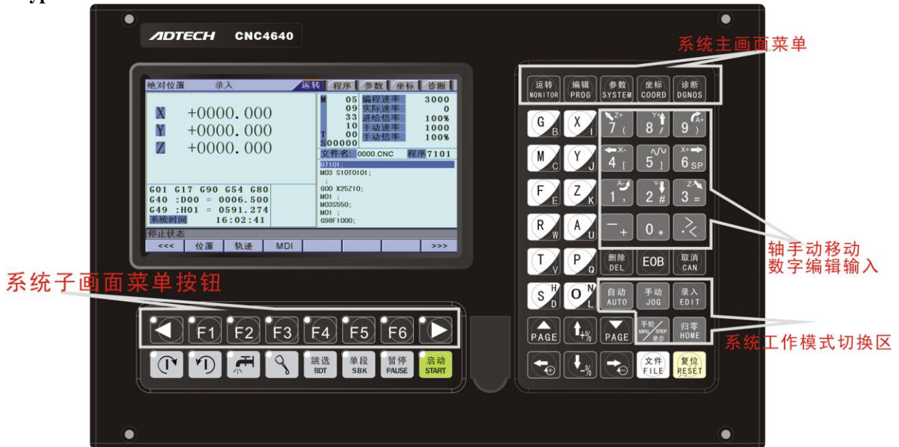
系统主画面菜单 Main screen of the system 轴手动移动 Manual moving of axis 系统工作模式切换区 System working mode switch section 系统子画面菜单按钮 Submenu buttons of the system 数字编辑输入 Number edit & input
